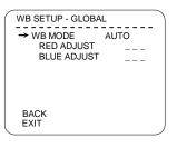
This menu allows the red and blue color levels to be adjusted automatically or manually.
